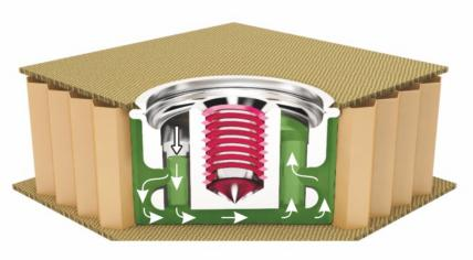
Fixing solutions using potted inserts are still widely used in sandwich panel structures.
